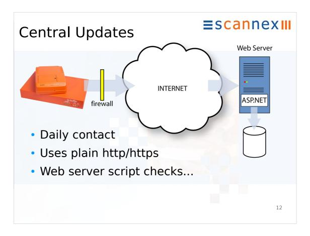
Rather than using VPN or other in-bound accesses to manage the remote buffers, the ip.buffer uses the standard HTTP mechanism to obtain updates.
